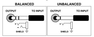
Fig. 3.12 Audio Output Wiring
